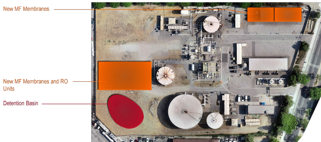
Figure 8-28. JMMCRWRP Single Pass RO Expansion – Scenario C Proposed Site Layout
